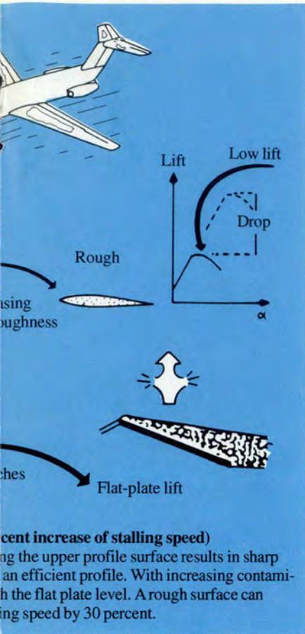
Generally, the better the wing is shaped, the larger the lift losses and drag increases due to surface contamination. Even mosquitoes deposited along a wing leading edge during summer operations have considerable effect on the stalling speed of some modern aircraft.
