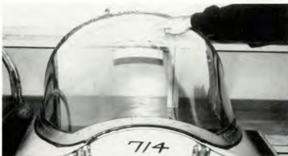
This is a new polycarbonate windscreen after being shot with a 4-pound chicken at 400 knots. No debris entered the cockpit.
