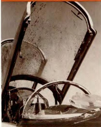
stand the impact of a 4-pound bird at 400 knots. The answer was a windscreen made of laminated polycarbonate. Unfortunately, since the new windscreen was designed to flex during bird impact, tests showed the brittle magnesium cast frame windscreen would break up, and the fragments could seriously injure the aircrew. Also, without the support of the frame, the windscreen would deflect and allow massive amounts of bird debris in the cockpit.
