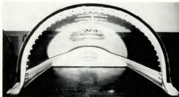
A pilot's view of the polycarbonate composite windscreen after a simulated bird strike.
