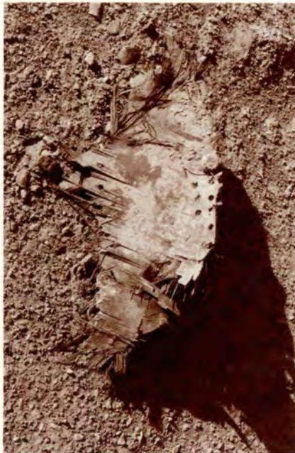
Composite panel showing post impact and heat damage with resulting released fibers.
