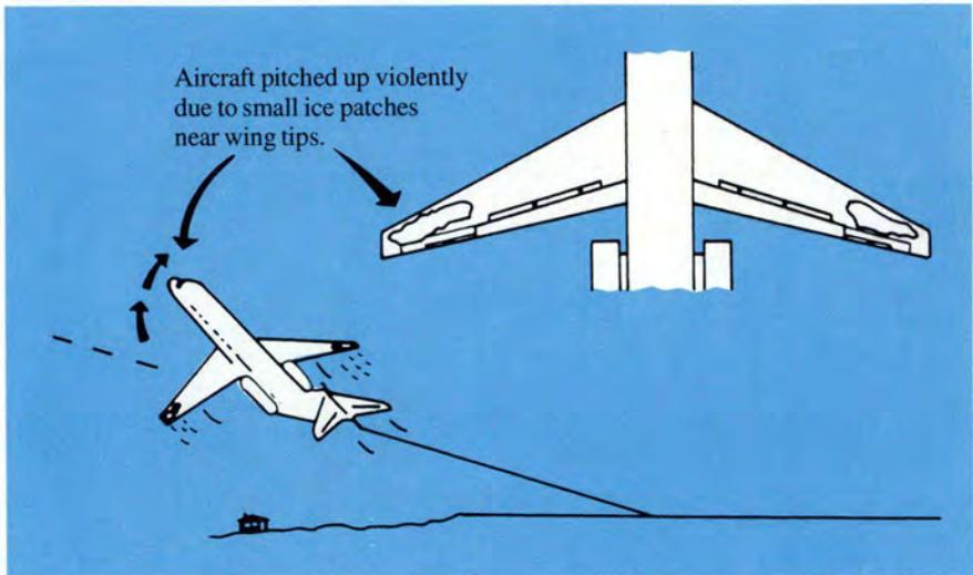
Aircraft stalled before stickshaker was activated due to contamination at wing leading edges
